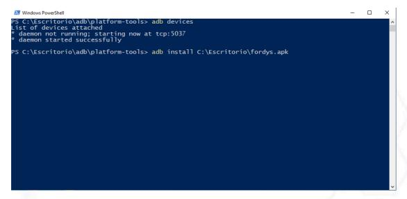
We check that our glasses are detected using "adb devices" and once verified we execute the command "adb install C: \ Desktop \ fordysVR.apk". After a few minutes fordysVR will have been installed on our device.
